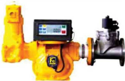
FCM-80-KPX-1 Meter with Electronic Register, Strainer, Air Eliminator & Solenoid Valve
